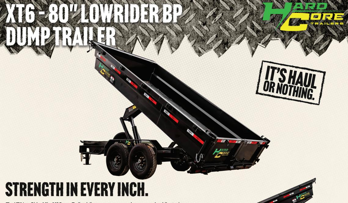
The XT6 LowRider 12' x 80" Dump Trailer delivers more space and more muscle while staying compact and maneuverable. With a 25" Easy-Access Deck, Ultra-Strong I-Beam frame, and HD QuickSlide™ 5'8" ramps, it's built for fast loading and dependable performance. Boasting a GVWR of 14,000 lbs and a load capacity of 10,274 lbs, the XT6 is the go-to choice for contractors, landscapers, and crews who need a trailer tough enough for daily heavy use yet sized right for any job site.
